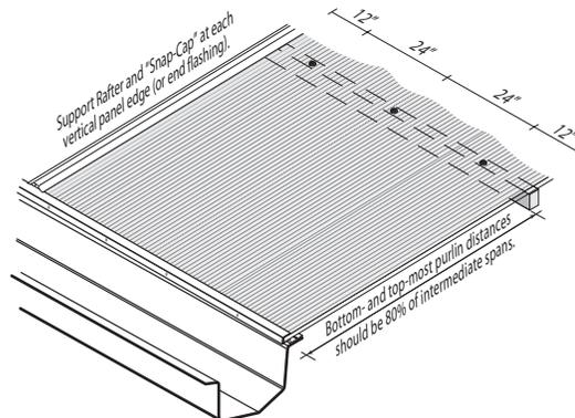
**At panel ends:** If panel ends are inserted into glazing profiles with channel recesses designed to accommodate polycarbonate (at ridge, gutter or eave), fasteners are optional, but are highly recommended when wind or snow loads can be excessive. If fasteners are used at these points, placement should be the same as at intermediate purlins.
